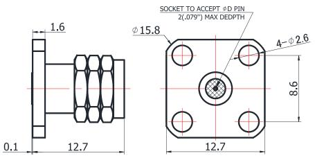
For glass-bead of 0.30mm pin diameter
