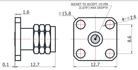
For glass-bead of 0.23mm pin diameter
