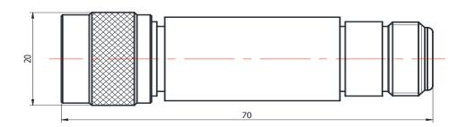
Dimensions refer to connector type N, Dimensions of other connectors are similar with Type N
