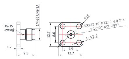
For glass-bead of 0.91mm pin diameter
