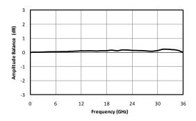
Fig. 3. Amplitude balance between output ports.
