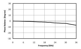
Fig. 4. Phase balance between output ports.
