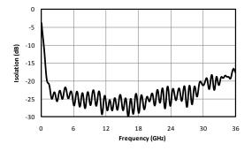
Fig. 5. Isolation between output ports.
