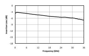
Fig. 1. Common port to output port insertion loss.
