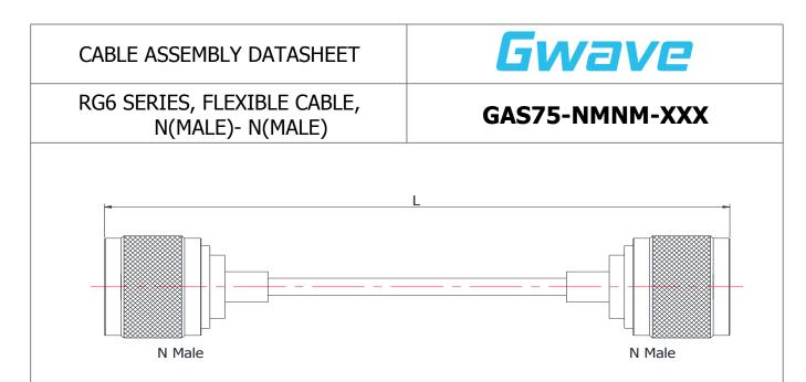
\* Label and Shrinking tube design depend on customer's request.
