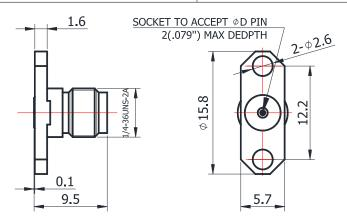
For glass-bead of 0.30mm pin diameter
