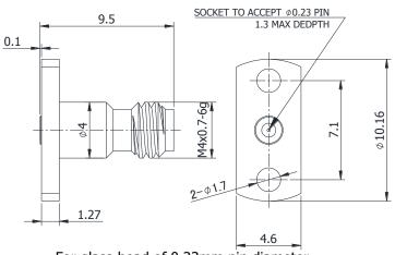
For glass-bead of 0.23mm pin diameter
