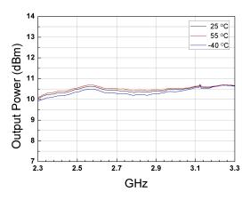
Figure.17 Output Power with -12dBm input power
