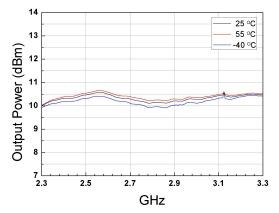
Figure.18 Output Power with -10dBm input power
