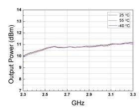
Figure 14 Output Power with -18dBm input power
