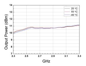
Figure.15 Output Power with -16dBm input power
