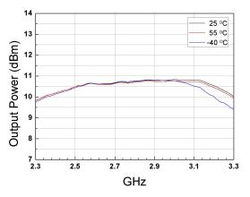
Figure.13 Output Power with -20dBm input power
